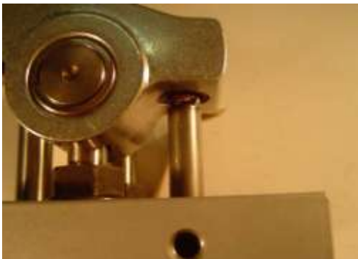
Correct Pushrod Fit 1.5 ratio Rocker
