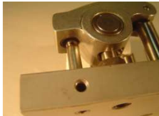
Incorrect Pushrod Fit for 1.5 Rocker
