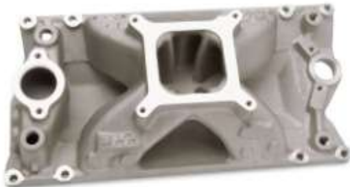
P/N 12366573 intake on the left is used on 602 engines. It's a dual plane, high rise intake. It has the 8 bolt Vortec mounting pattern.
