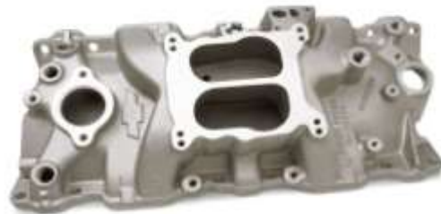
P/N 10185063 intake on the right is used on 603 engines. It is a dual plane medium rise style. It uses 12 bolt traditional mounting.
